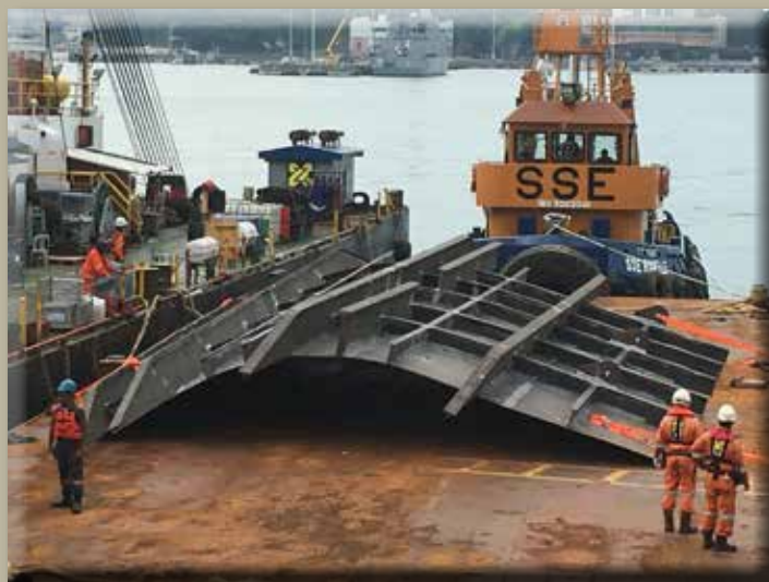
The completed patch being positioned next to USS JOHN S MCCAIN for installation.
