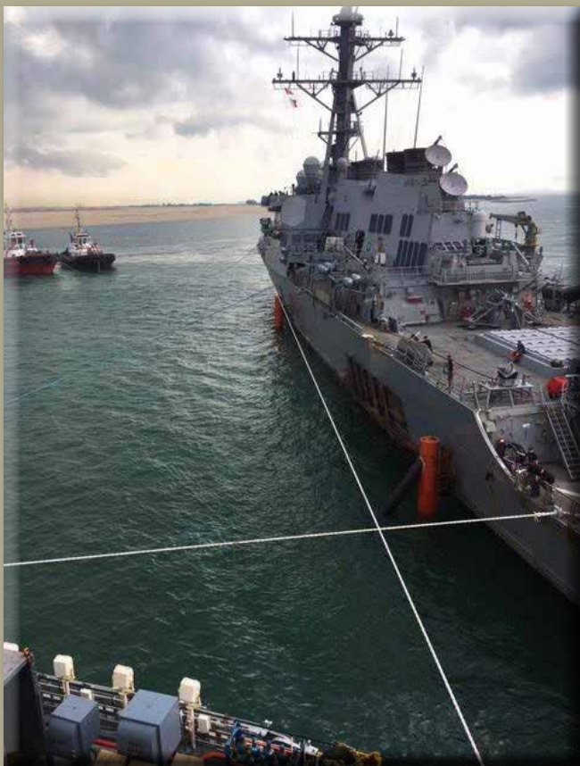
USS JOHN S MCCAIN positioned on the alignment posts which have been welded to the deck of heavy lift ship TRESSURE. In this picture, divers had verified the keel was sitting correctly on the blocks and deballasting has begun.
