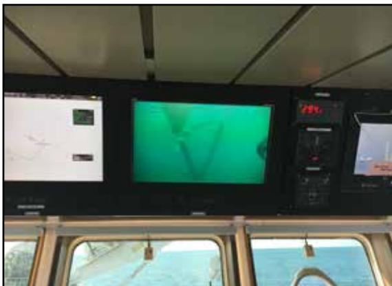
Display of ROV footage of main hook pendant suspended in water column by lift bags.
