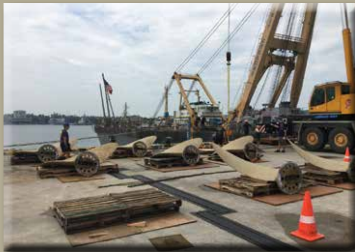
Seven of JOHN S MCCAIN's propeller blades removed from the hub. The sheerleg crane, CYCLONE, is shown in the background supporting patch installation.
