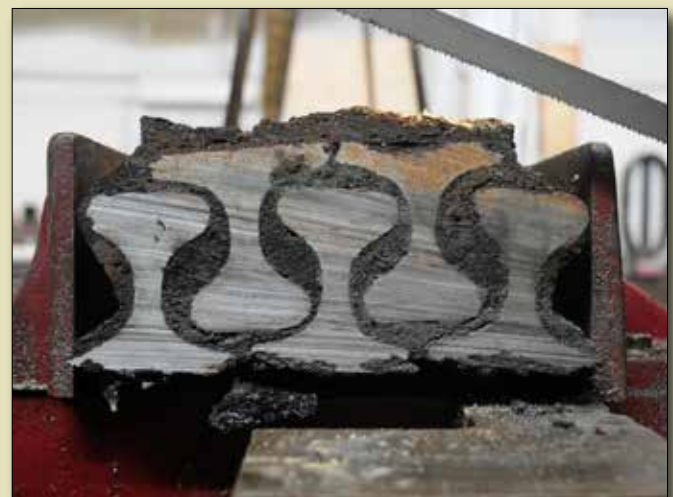
Cross-section of Armor from CSS GEORGIA test Casemate Section.
